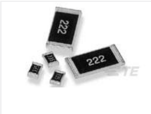
TE Part #5-1879497-7 CRGH1206 5% 220R 0.5W
