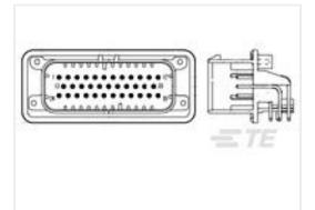
TE Part #1-776163-6 35POS,PIN DIA 1.3,HDR ASSY,90DEG, COD 6
