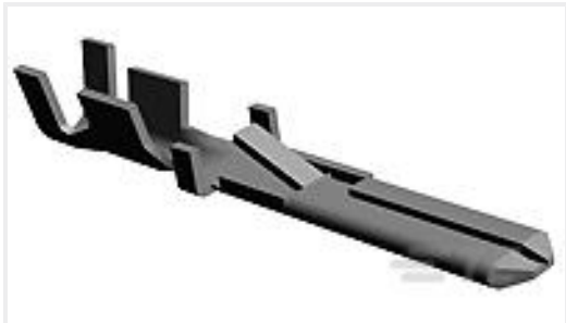
TE Part #928931-2 FF 110 (2.8 X 0.8 MM) TAB PTP CUZN30
