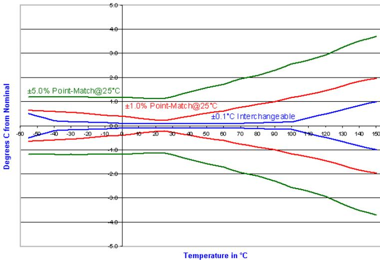
This chart compares the tolerance differences between an interchangeable thermistor and two point-matched thermistors.
