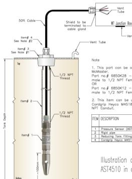
This part can be order from McMaster. Part no.# 6850K28 - 1.5" NPT male to 1/2 NPT Female Part no.# 6850K12 - 2" NPT mole to 1/2 NPT Female.
