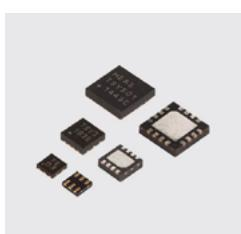
**Digital temperature sensors** integrate sensing elements, signal conditioning, and analog-to-digital conversion within a single microcircuit.
