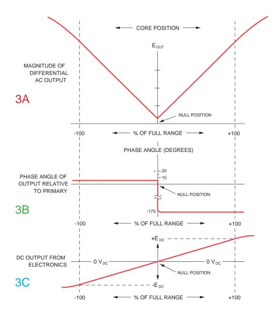
FIGURE 3: THE OUTPUT CHARACTERISTICS OF AN LVDT VARY WITH DIFFERENT POSITIONS OF THE CORE. FULL RANGE OUTPUT IS A LARGE SIGNAL, TYPICALLY A VOLT OR MORE, AND OFTEN REQUIRES NO AMPLIFICATION. NOTE THAT AN LVDT CONTINUES TO OPERATE BEYOND 100% OF FULL RANGE, BUT WITH DEGRADED LINEARITY.
