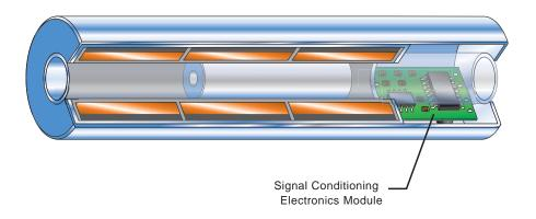
FIGURE 4: THE CROSS SECTIONAL VIEW OF THE DC-LVDT AT LEFT SHOWS THE BUILT-IN SIGNAL CONDITIONING ELECTRONICS MODULE. THE MODULE IS SECURED WITH A POTTING COMPOUND THAT IS NOT SHOWN IN THIS DRAWING.
