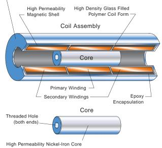
FIGURE 1: THE PRIMARY WINDING IS ILLUSTRATED IN THE CENTER OF THE LVDT. TWO SECONDARY COILS ARE WOUND SYMMETRICALLY ON EACH SIDE OF THE PRIMARY COIL AS SHOWN FOR "SHORT STROKE" LVDTS OR ON TOP OF THE PRIMARY COIL FOR "LONG STROKE" LVDTS. THE TWO SECONDARY WINDINGS ARE TYPICALLY CONNECTED IN "SERIES OPPOSING" (DIFFERENTIAL).
