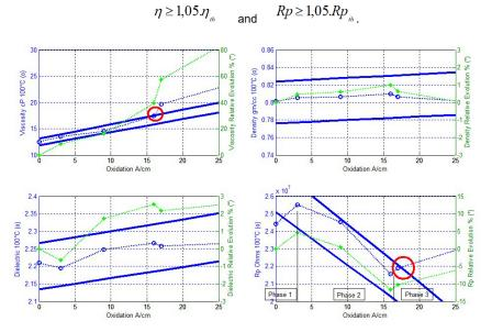
FIGURE.2.3: ENGINE OIL (15W40) OXIDATION MEASURED BY FPS2800 AT 100°C
