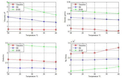
FIGURE.2.8: GASOLINE, DIESEL BO, RAPESEED B100 BIODIESEL MEASURED BY FPS2800
