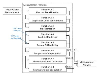
FIGURE.3.2: MEASUREMENT FILTRATION BLOC DIAGRAM 1
