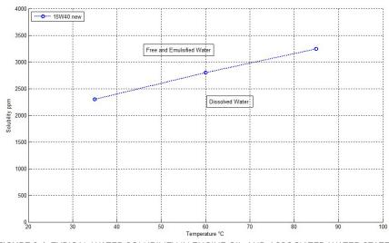
FIGURE.2.4: TYPICAL WATER SOLUBILITY IN ENGINE OIL AND ASSOCIATED WATER STATES
