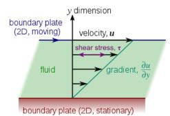
FIGURE.1.4: SHEAR STRESS OF FLUID BETWEEN TWO PLATES
