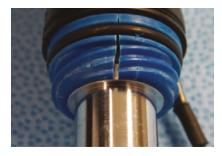
Fig.1. Mechanical stresses, like threaded mating components, can increase likelihood of cracking due to reprocessing.
