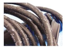
Fig.3. Blooming of Additives after repeated  $H_2O_2$  Sterilization.
