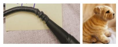
Fig.4. "Shar Pei" effect-stretching of cable jackets due to repeated manual cleaning
