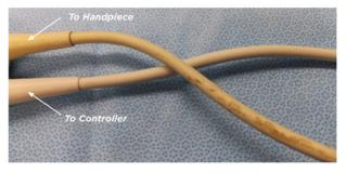
Fig.5. Cleaning/disinfection can lead to discoloration
