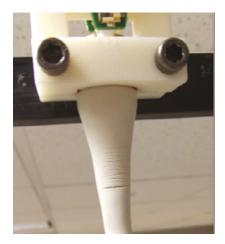
Fig.2. Cracking of a cable flex relief due to combination of cleaning + handling.
