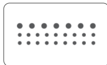
25 Position 18 * AMP MCP 1.5K + 7 * AMP MCP 2.8
