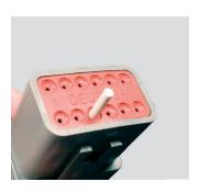
Apply pressure until sealing plug locks into place. A slight tug on the sealing plug will confirm it is locked into place.
