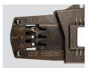
**Step 1:**Cycle the hand tool to the open position. Place the contact into the correct die nest.
