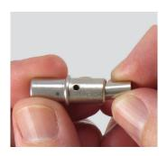
**Step 1:**Place crimp sleeve reducer into contact barrel.
