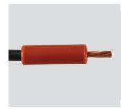
Step 2: Slide insert seal onto 8-10 AWG wire stopping just at the edge of the stripped insulation.
