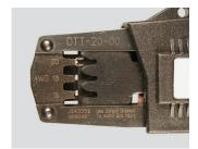
**Step 2:**Partially close the tool until the contact is held in place.
