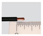
**Step 3:** Measure the exposed strands to be sure the crimp length is correct.
