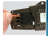
**Step 3:** Insert the prestripped wire into the crimp area of the contact.
