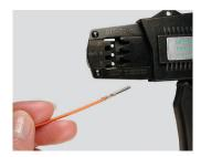
Close the tool until the ratchet releases. The ratchet is released when a loud click is heard and crimp is complete.
