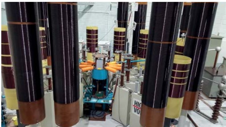
High energy surge arrester test system
