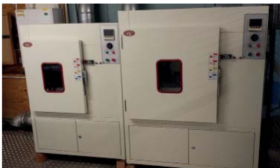
HV varistor block ageing test system with AC and DC supply
