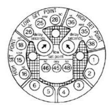
The delay circuits drive double pole double throw output relays. LED's mounted on the front fascia show the operational state of the relays.
