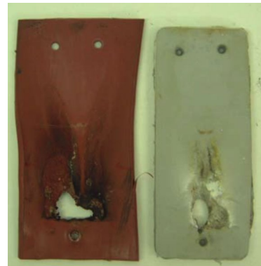
Failure by erosion
