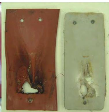
Failure by erosion
