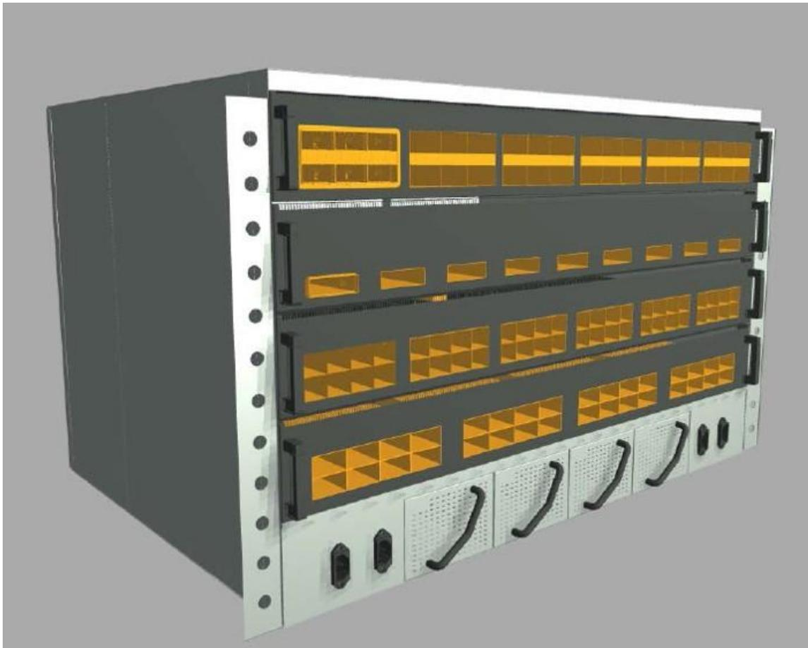
Modular equipment showing various 1RU line cards with 36, 9, 48 and 32 ports
