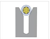
As insertion begins, the wire insulation is displaced.
