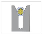
Insulation displacement is completed and conductor strands begin to deform.
