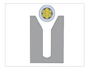
The wire must be aligned with the IDC slot
