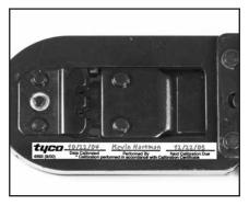
A label conveniently located on the crimp head, which moves with the head from tool to tool, lets the operator see when certification or inspection is due.
