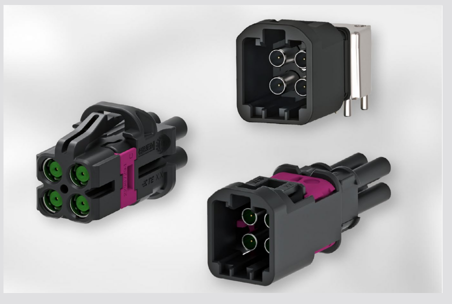
Fig. 2: MATE-AX initial product offering: 90° header, 180° inline connector, and 180° plug connector (from left to right)
