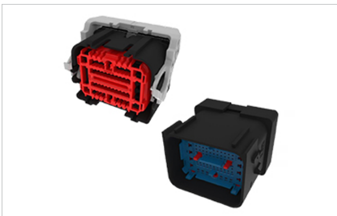
Figure 3: Generation Y 68P Sealed Hybrid Inline Connector. Generation Y 0.64 mm and MATE-AX Mini Coax Connector for applications where separate low voltage power and signal connectors run alongside traditional data connectivity. Typical applications include high-resolution cameras and displays, antenna connections, transfer of video and sensor signals. Learn more.
