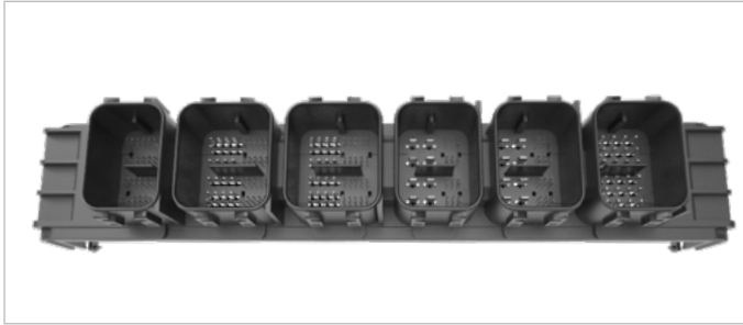
Figure 2: 254 Position hybrid header for an engine management ECU: 160 x NanoMQS (0.5 mm), 78 x MCON 1.2 mm, 16 x AMP MCP 2.8 mm (example).
