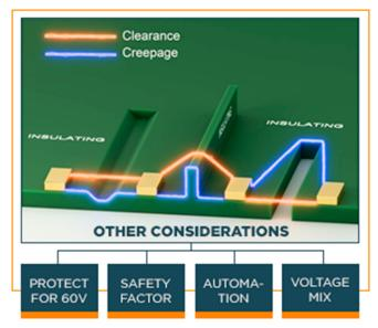
connectors that address a wide range of application needs. This standardized 48V LVCS product family are designed to maximize packaging efficiency and scalability, while meeting stringent creepage and clearance requirements.
