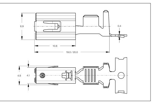
**Contact Resistance:** New State  $\leq 2 \text{ m}\Omega$ Mating Cycles: up to 10 cycles (tin plated) up to 50 cycles (silver plated) Mating Force: Max. 12 N Unmating Force: Max. 11 N **Extraction Tool:** Part No. 1-1579007-3
