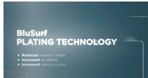
TE Connectivity (TE's) innovative BluSurf plating technology is now available for use with TE's MCON 1.2 12P-24P sealed inline connector system with TE's mono clean body contact systems, providing automotive manufactures reduced mating force by (up to 40% lower than standard terminals), increased durability and mating cycles and improved insertion force.
