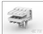
3P, PCB Locking Wire-To-Wire, Insulation Displacement, PA 6 GF, Fully Loaded 1-1740501-3
