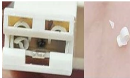
Example Part: FASTON 250 Receptacle P/N 1969295-4 Skiving of Plastic Housing
