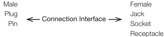
Figure 2. Typical RF Coaxial Connector Gender Terms
