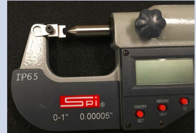
SPECIAL FIXTURE FOR 2D CRIMP MEASUREMENT
