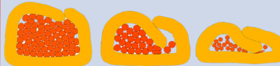
BAD WIRE BARREL CRIMP CROSS SECTION
