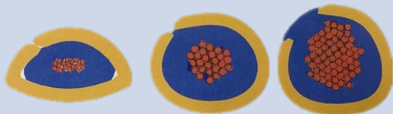
GOOD INSULATION BARREL CROSS SECTION
