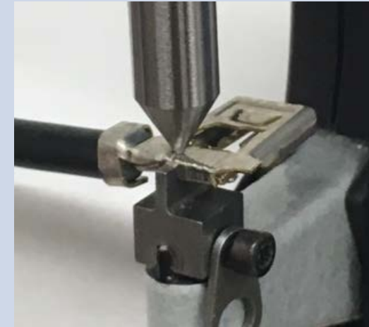
SPECIAL FIXTURE FOR 2D CRIMP MEASUREMENT
