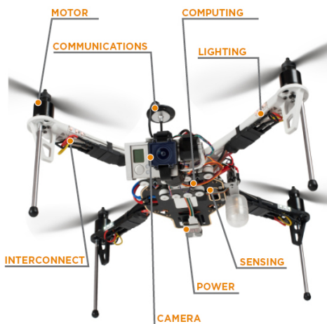
Subsystems of Commercial Drones.
