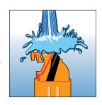
Protected against powerfully jetting water with increased pressure (Automotive)
