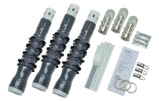
TE's Raychem Cold Shrink Terminations CSTI/O are made from a high performance, liquid silicone material which is specially formulated for excellent tracking and split resistance. The extra-long silicone stress cone is integrated within the termination which ensures correct positioning. Moisture sealing at the lug is integrated into the termination body, eliminating the need for additional sealing tapes.
