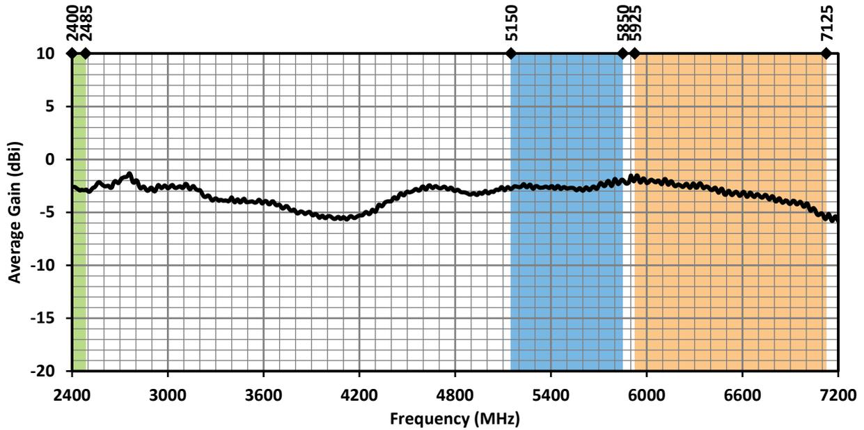
Figure 6. ANT-W63-MSA-TH1 Average Gain with Frequency Band Highlights
