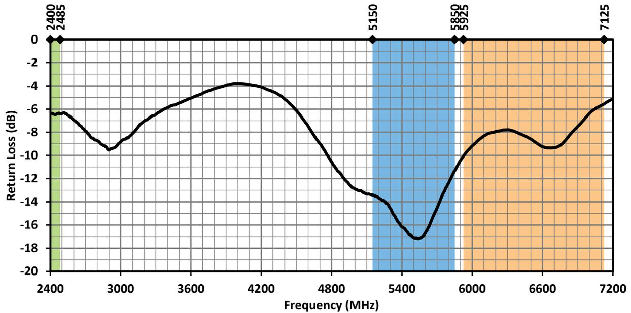
Figure 4. ANT-W63-MSA-TH1 Return Loss with Frequency Band Highlights
