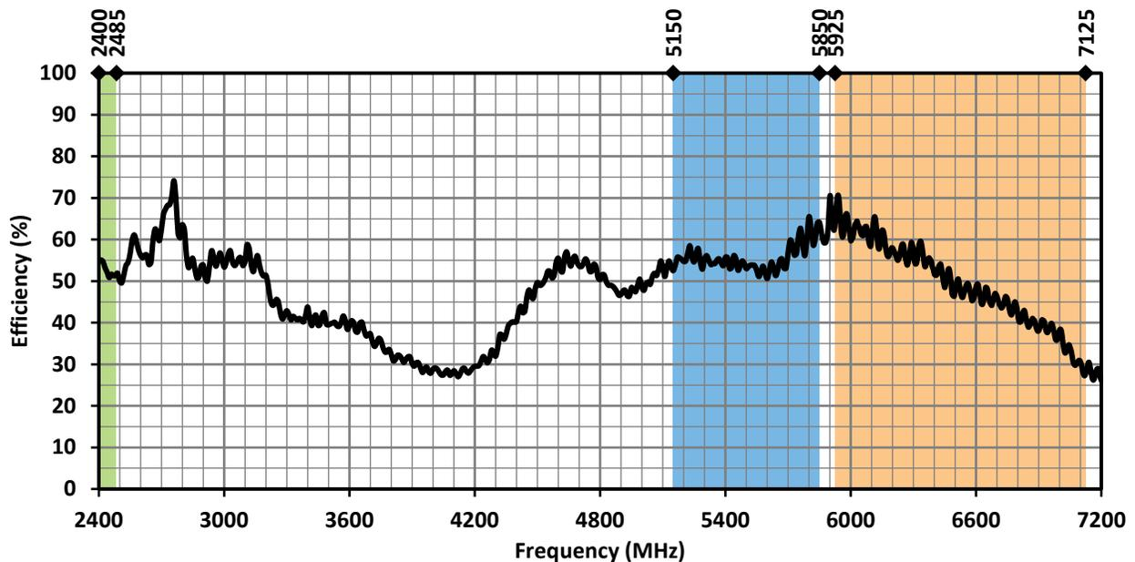
Figure 7. ANT-W63-MSA-TH1 Radiation Efficiency with Frequency Band Highlights
