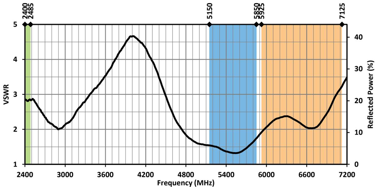
Figure 3. ANT-W63-MSA-TH1 Antenna VSWR with Frequency Band Highlights
