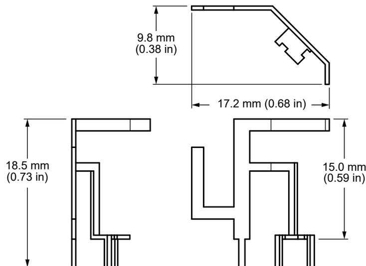
Figure 1. ANT-W63-MSA-TH1 Antenna Dimensions
