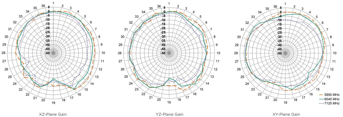
Figure 8. ANT-W63-MSA-TH1 Antenna Radiation Patterns
