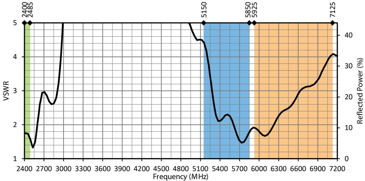
Figure 12: ANT-DB1-WRT-ccc VSWR, at Center of Ground Plane
