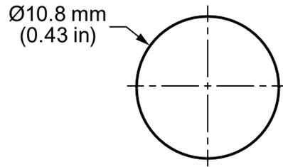
Figure 2: ANT-DB1-WRT Series Antenna Recommended Enclosure Mounting Dimensions
