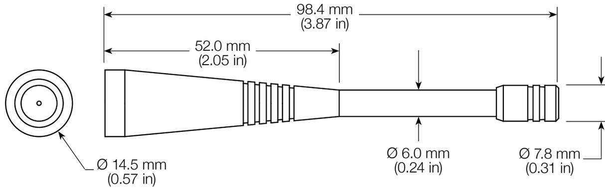
Figure 6: CW LTE Band 28 Antenna Dimensions
