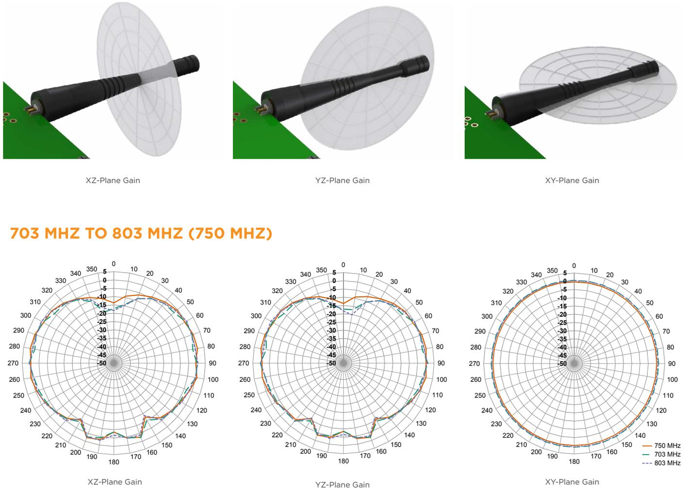
Figure 8: Radiation Patterns for CW LTE Band 28 Antenna
