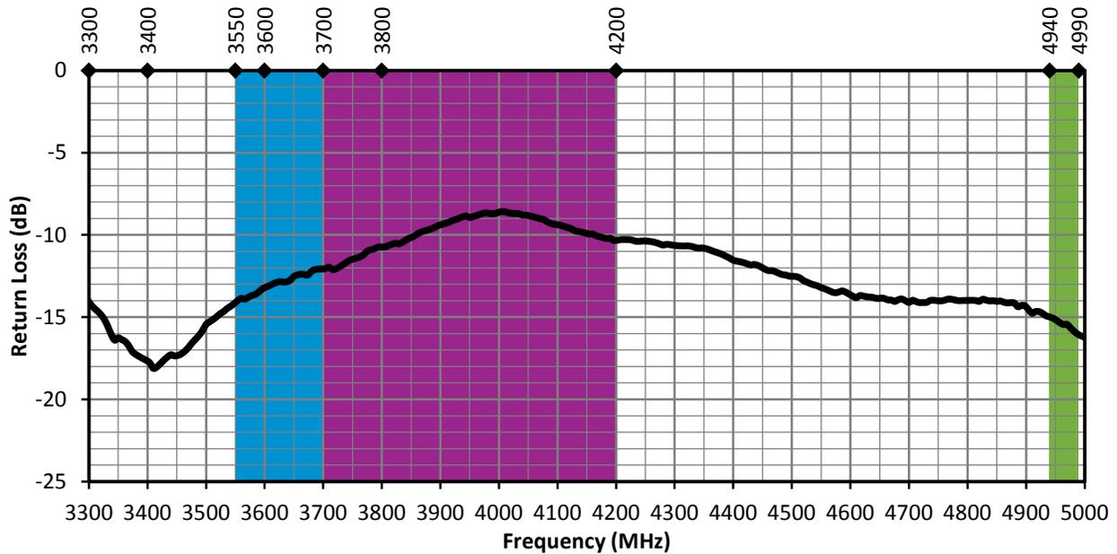
Figure 12. 5GMWP1 Return Loss, Edge-Bent
