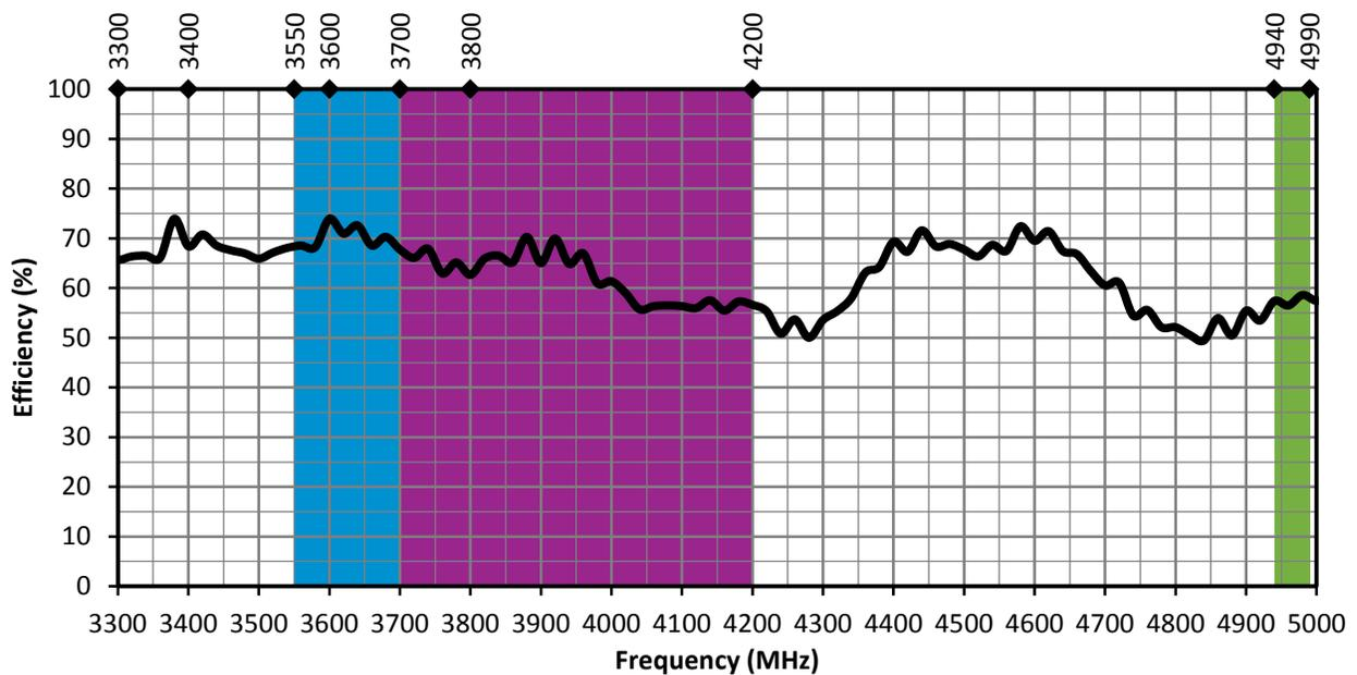
Figure 15. 5GMWPI Antenna Efficiency, Edge-Bent
