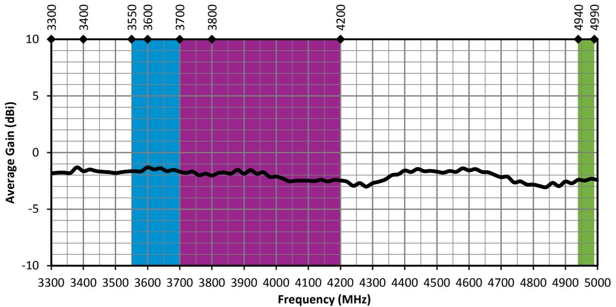
Figure 14. 5GMWPI Average Gain, Edge-Bent
