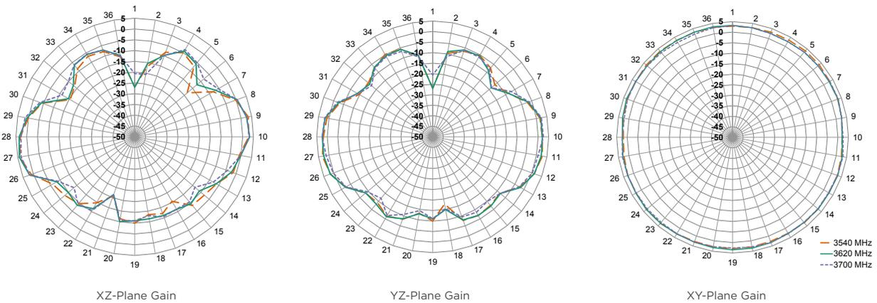
Figure 16. Antenna Radiation Patterns for the 5GMWP1, on Edge of Ground Plane, Bent at 90 Degrees
