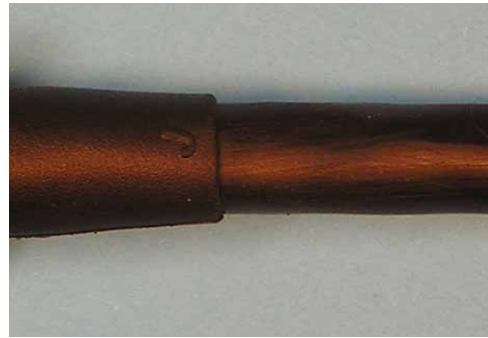
NOT ACCEPTABLE insufficient adhesive flow /180
