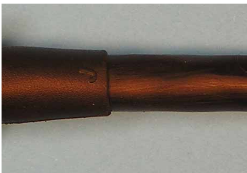
NOT ACCEPTABLE Insufficient adhesive flow /42, /86
