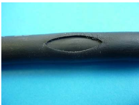
NOT ACCEPTABLE Tubing Split
