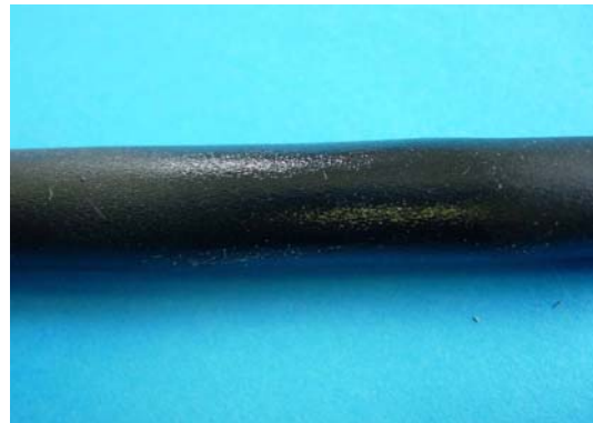
NOT ACCEPTABLE Tubing scorched
