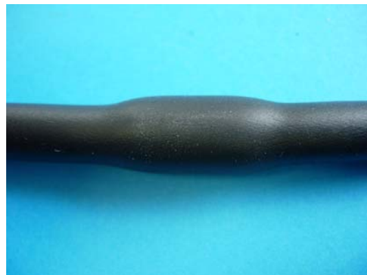
NOT ACCEPTABLE Air entrapment or tubing not fully recovered
