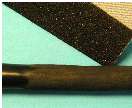
Figure 1 Degreased and abraded cable jacket
