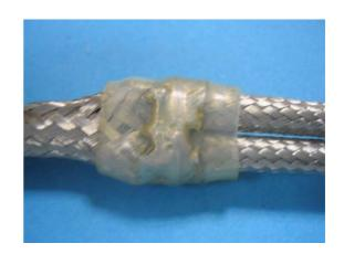
Figure 5B Insufficient Solder Flow
