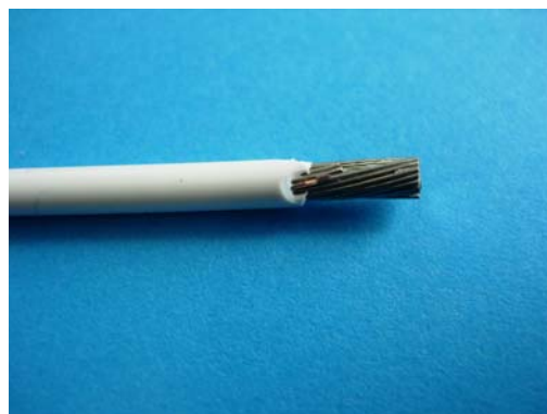
NOT ACCEPTABLE Damaged and nicked conductors
