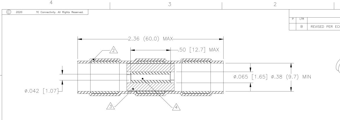
MATCHED IMPEDANCE SPLICE FOR RG400 & RG142 COAXIAL CABLE REPAIR
