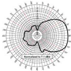
Azimuth Pattern (X, Y, or E-plane)
