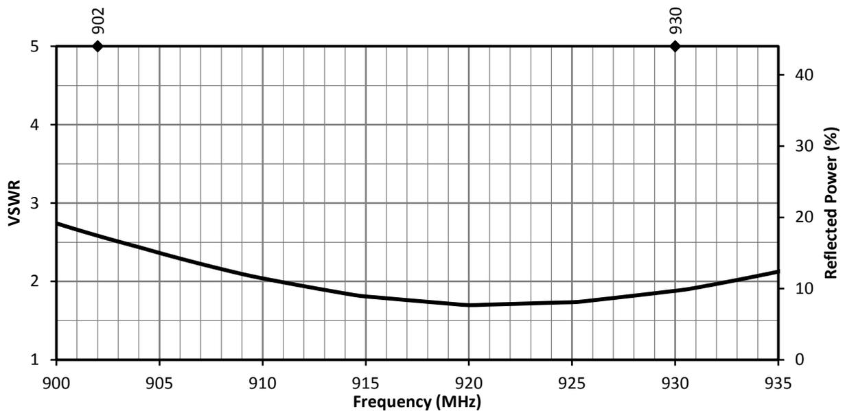
Figure 4. VSWR for ANT-915-NUB-ccc, Edge of ground Plane
