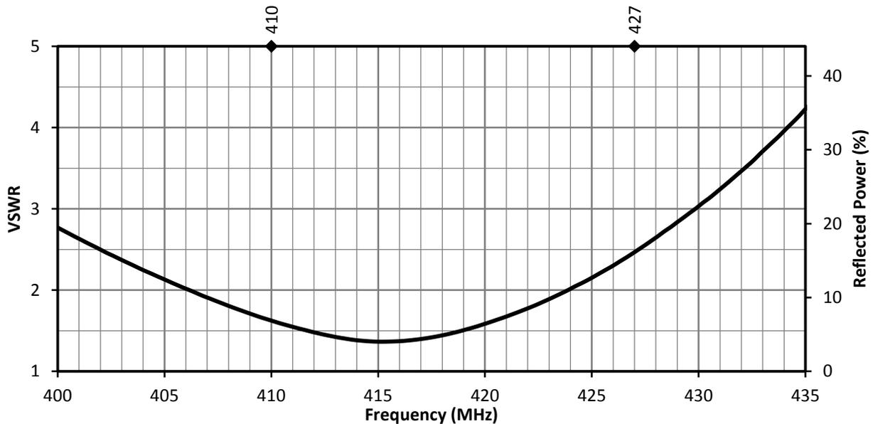
Figure 12. ANT-418-WRT VSWR, at Center of Ground Plane
