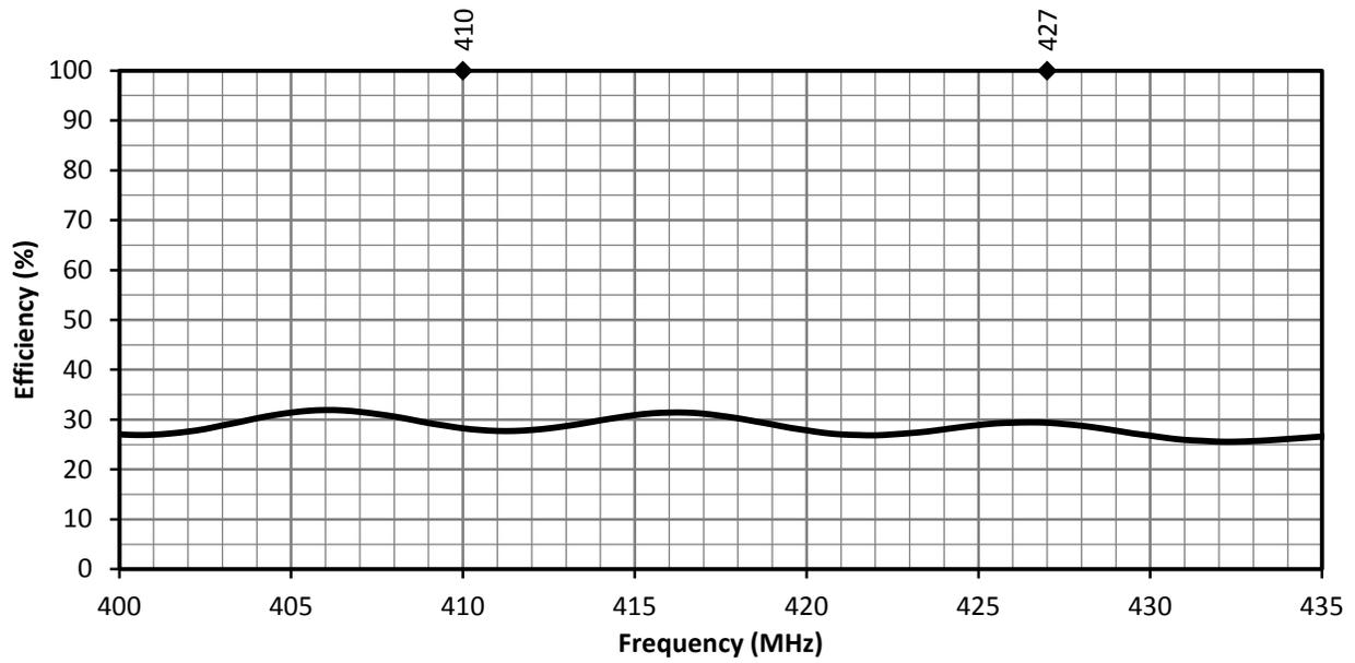
Figure 9. ANT-410-WRT Antenna Radiation Efficiency, Free Space
