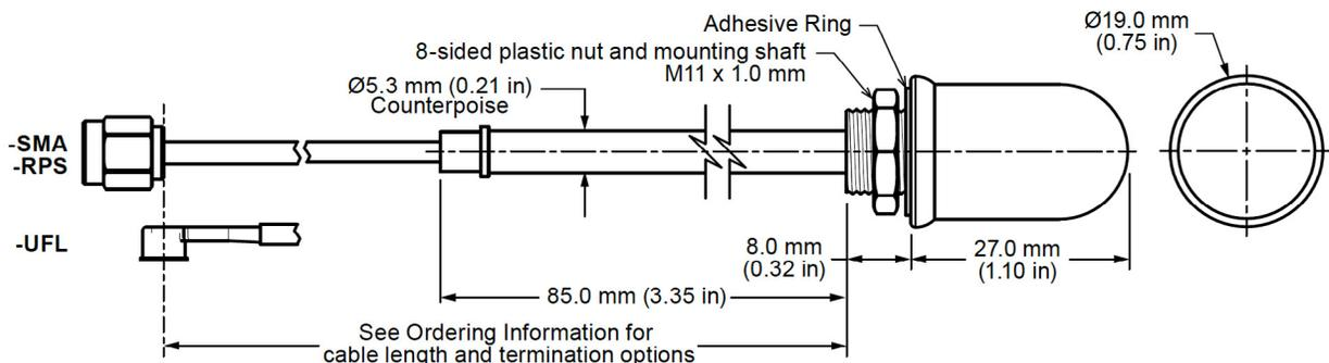
Figure 1. ANT-410-WRT-ccc Antenna Dimensions
