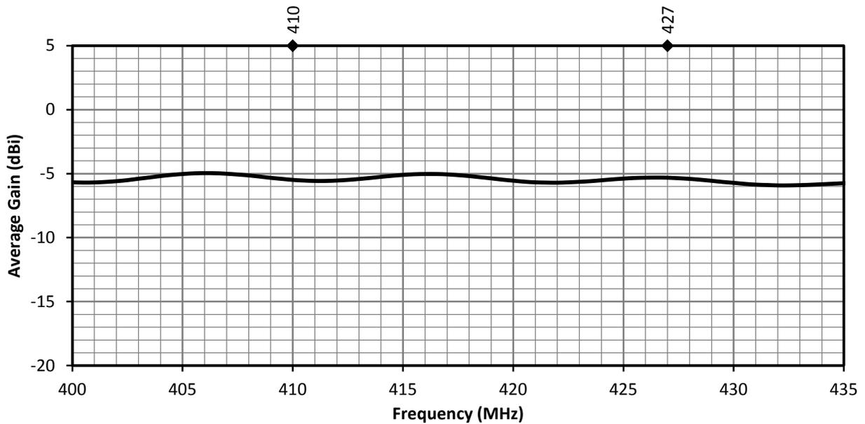
Figure 8. ANT-410-WRT Antenna Average Gain, Free Space
