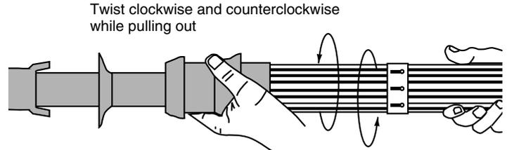
Using the pull tabs, pull the flip-back portion away from the main termination, at the same time working the first two fingers of each hand between the flip-back and main termination. Pull the stretched out flip-back over the cable jacket and sealant.
