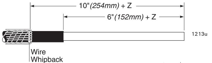
**Z=Depth of lug's Barrel + "X" Expansion Gap**
