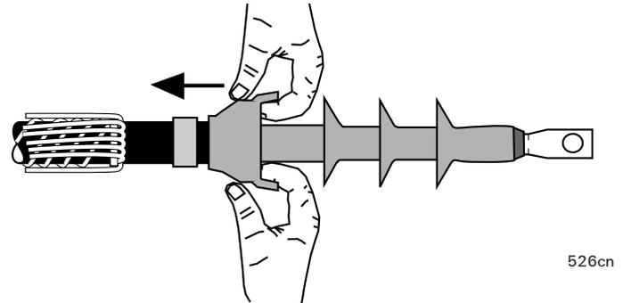
Wipe over the surface of the termination to remove any dirt or grease.
