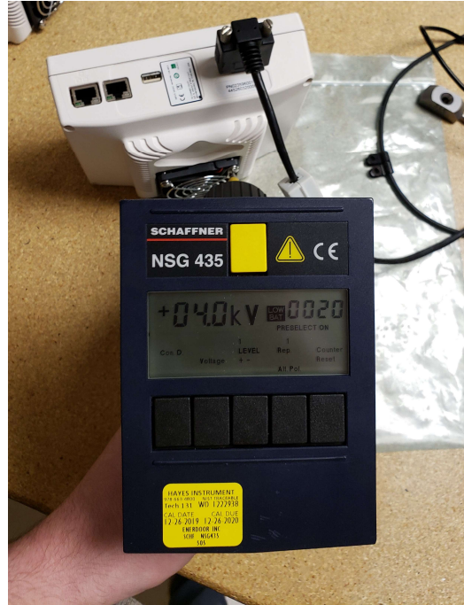
Photo 6: Electrostatic Discharge Immunity. Contact Discharge Test Point C2.
