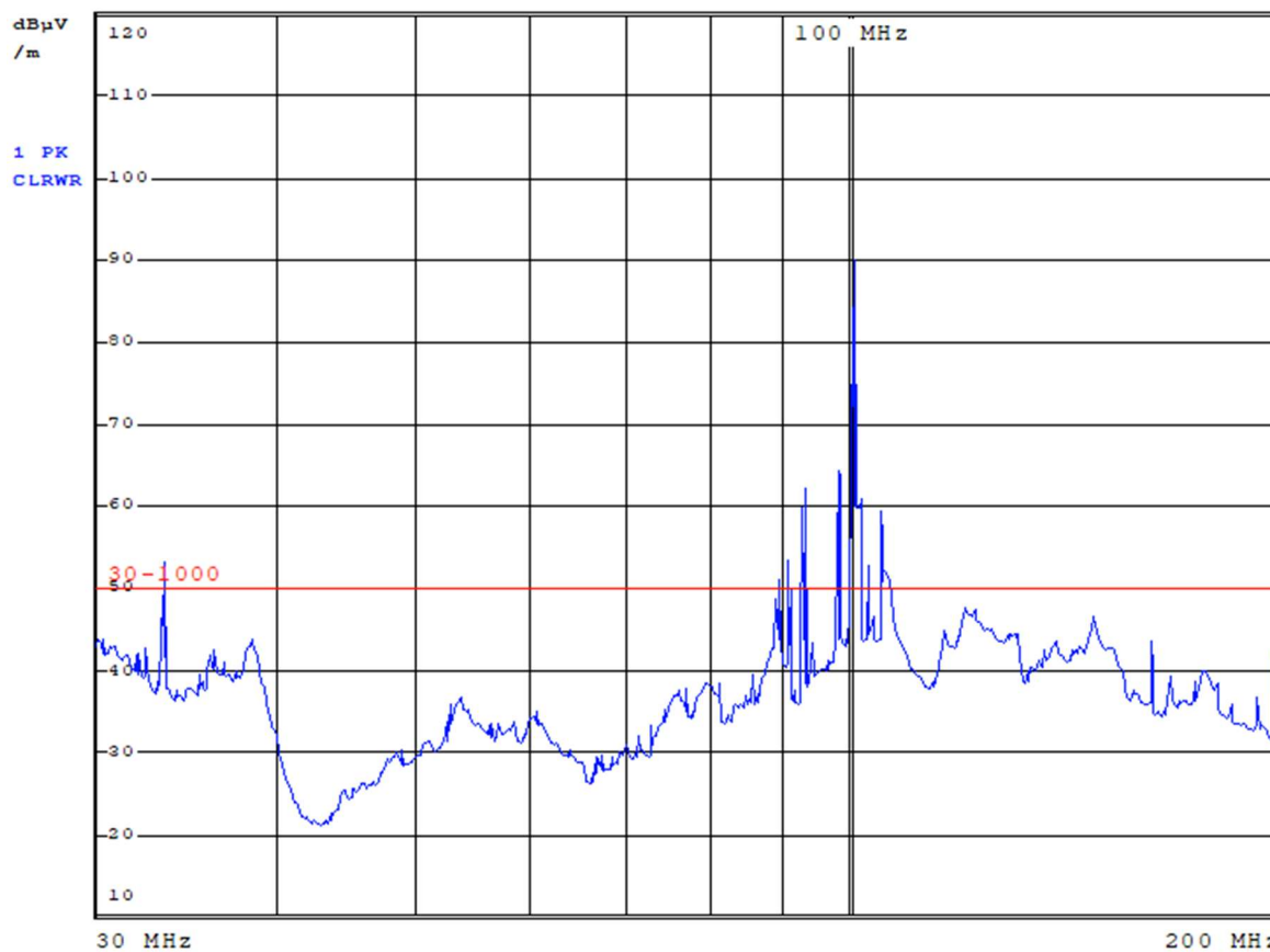
Graph 7: Machine Off. Ambient Noise. Radiated Emissions. Biconic Antenna. Horizontal Polarization. Revision A.
