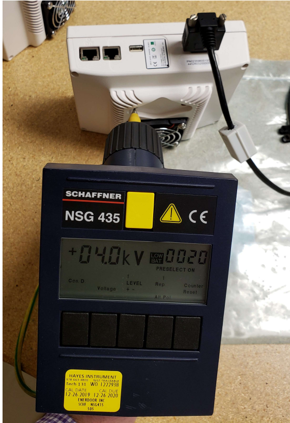
Photo 7: Electrostatic Discharge Immunity. Contact Discharge Test Point C3.
