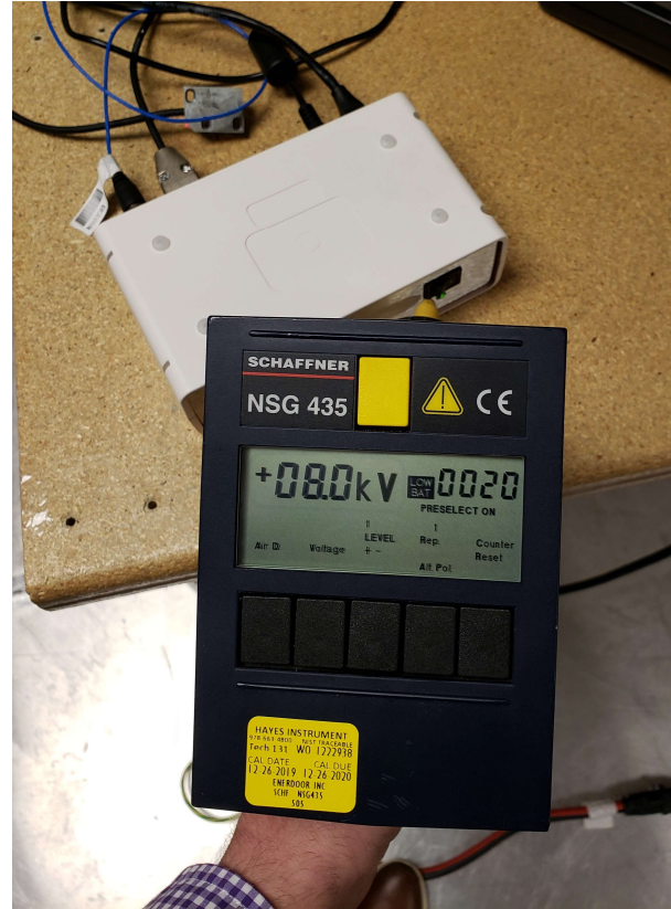
Photo 8: Electrostatic Discharge Immunity. Air Discharge Test Point A1.
