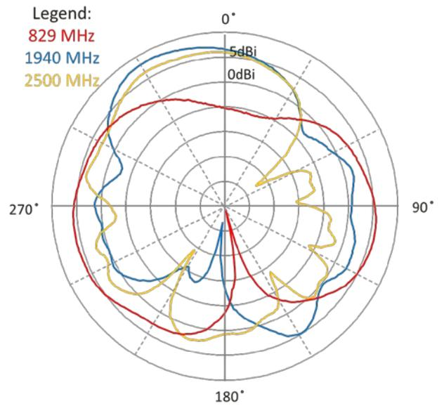
Data measured in free space and on plastic device enclosure
