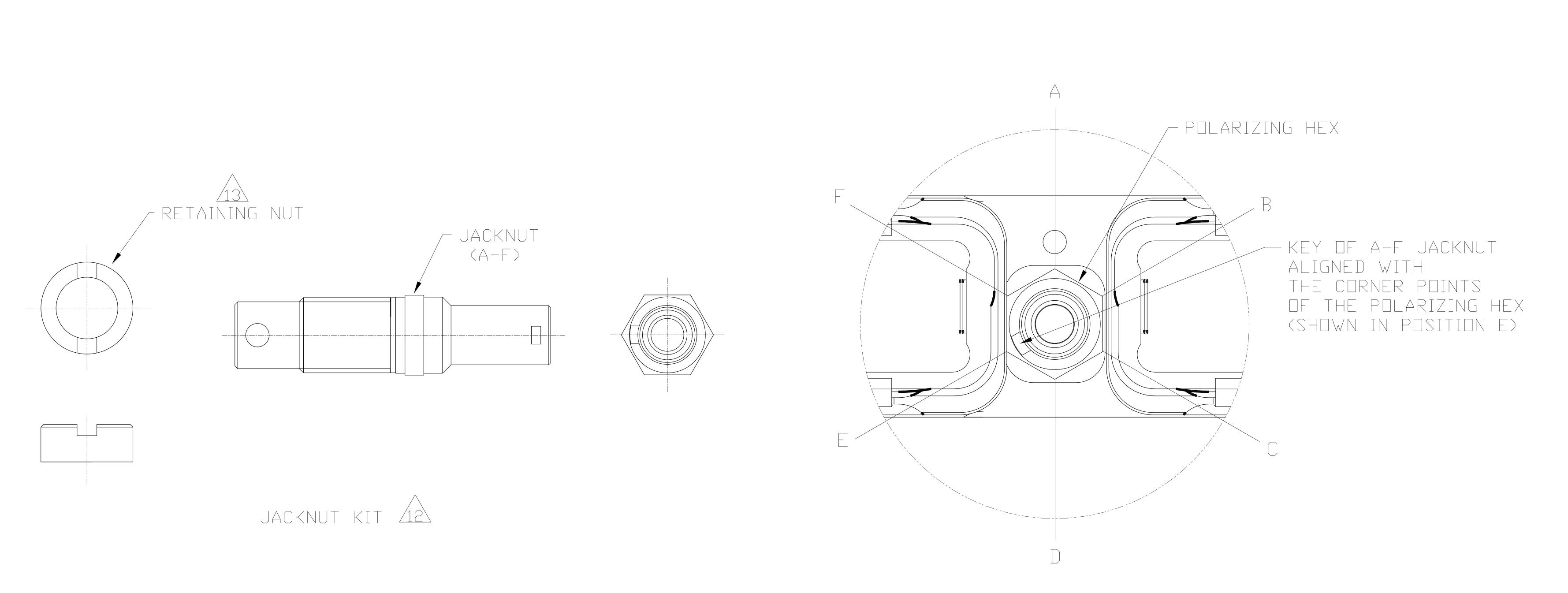
DETAIL A - JACKNUT KIT ASSEMBLED
