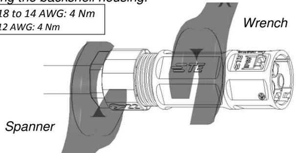
Figure 7, In-Line connector preparation
