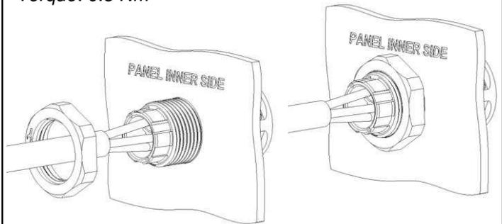
Figure 8, Panel Mount connector preparation
