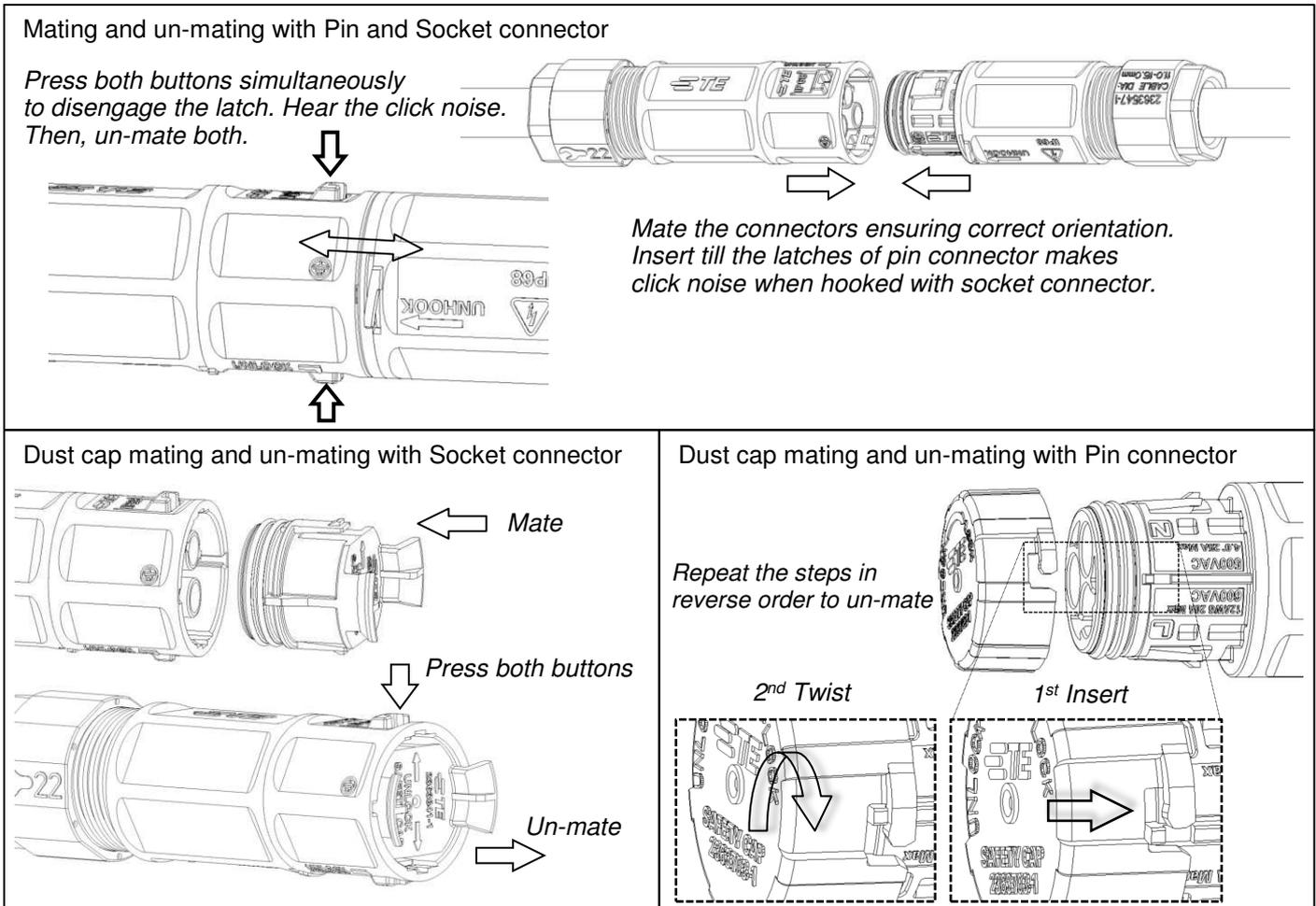
**Figure 9, Mating & Un-mating function**
