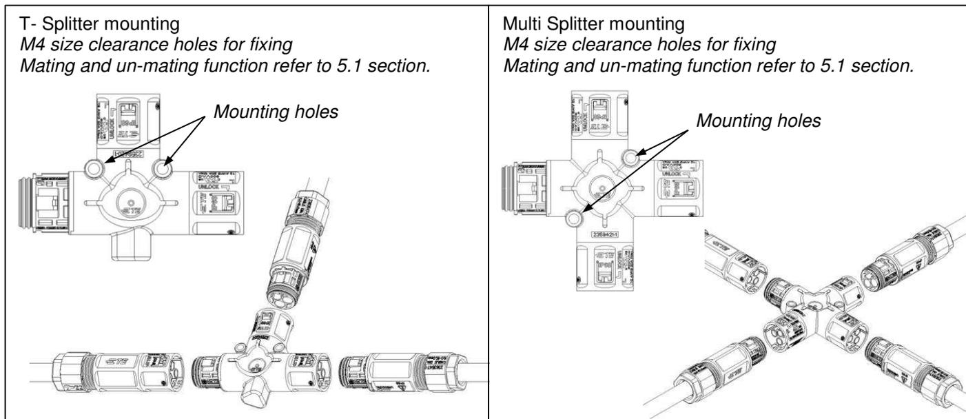
Figure 11, Splitter mounting
