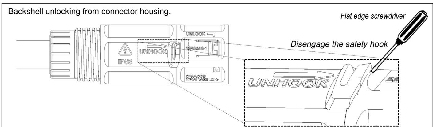
**Figure 10, Backshell un-locking**
