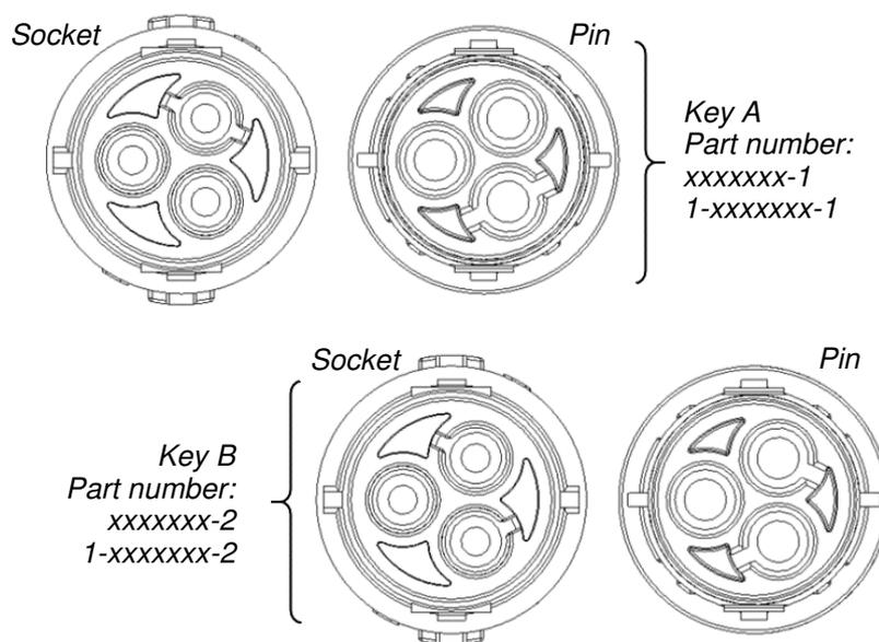
**Figure 4, Polarization keys**
