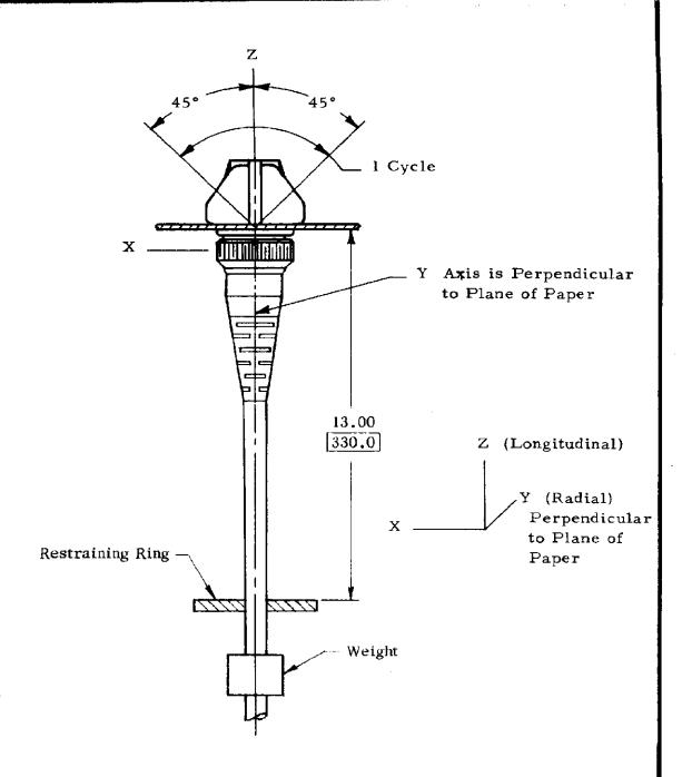
Note: Samples shall be conditioned in air circulating oven at a temperature of  $105^{\circ}\text{C}$  for 24 hours. Samples shall then be cooled for one-half hour maximum, at ambient, before test.
