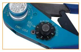
**2** Set the dial of the crimp to the proper setting for wire gage and contact as noted on the contact information sheet or on the tool. Be sure that the proper locator is used. See contact information sheet for proper locator.
