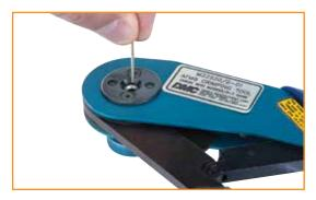
**3** Drop the contact into the crimping tool with the contact crimp barrel facing up.
