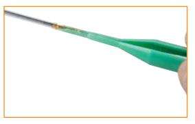
**2** After the wire snaps into the tool, seat the retention shoulder against the tip of the tool.
