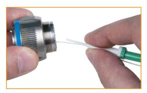
1 With the rear of the connector facing you, lay the wire of the contact along the slot of the tool, leaving about 1/2" from the end of the tool to the rear of the connector. Squeeze the wire firmly into the tool between the thumb and forefinger about 1/2" from the tip and quickly pull the tool away from the connector.
