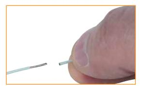
**4** Remove the small piece of insulation from the wire. Do not pinch the insulation with the fingernails during this procedure. The wire is now ready to be crimped to the contact.
