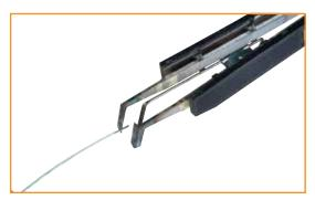
1 Burn through the insulation with a hot wire stripper or use other approved stripping method. Do not remove the insulation at this point. This will help protect the wire strands from splaying. Refer to contact information sheet for proper wire insulation strip length.
