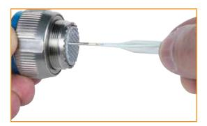
**3** Press the wire of the contact against the serrations of the plastic tool and pull both the tool and the contact/wire assembly out of the connector.
