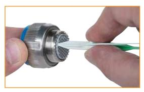
**2** The wire will now have snapped into place. Slide the tool down along the wire and into the rear cavity and slowly into the connector until a positive resistance is felt. At this time, the contact retaining mechanism is in the unlocked position.
