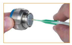
**3** Holding the connector with the rear grommet facing you, slowly push the contact straight into the grommet cavity. Do not twist the tool. Note: Some wire constructions may not require the use of an insertion tool.
