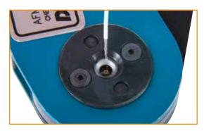
**5** Insert the bare wire into the open end of the contact and squeeze the handles of the tool together. The crimping tool will not release until the full crimping cycle has been performed. Remove the crimped contact and wire from the tool.
