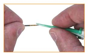
**1** Hold the insertion half of the tool between the thumb and forefinger and lay the wire against the slot of the tool, then snap the wire into the slot.
